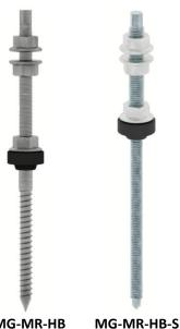
Hanger Bolt apply to install on both wooden rafter and steel purlin. Both types can be applied with L Foot and plate. There are three sizes most common use, M10x200mm, M12x200mm and M12x300mm Hanger bolt.
