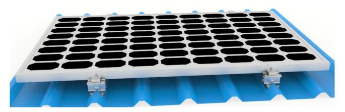
Universal Roof Clamp can work with all kinds of trapezoidal metal roof. It is a rail-less solution, it will help you save some cost and labor cost. Use anti-aging EPDM rubber to improve the waterproof performance. The material of this product is made by aluminum alloy (AL 6005-T5) and stainless steel 304 (SUS 304), which has strong corrosion resistance.
